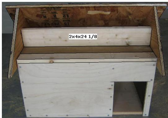
**Step 2, Assemble the Base** - Select the Bottom, the Front, Back, Divider, Top Braces, and two Side panels; attach them with 1 5/8" screws as shown above (pre-drill and counter sink each screw hole).
